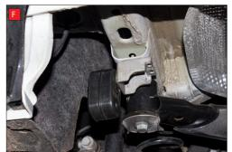
A) After you have removed O.E exhaust you will need to swap the valve motors to the Scorpion exhaust. Remove the 3 nuts ( keep safe as you will need them to bolt the electronic valve motor to Scorpion Exhaust).
